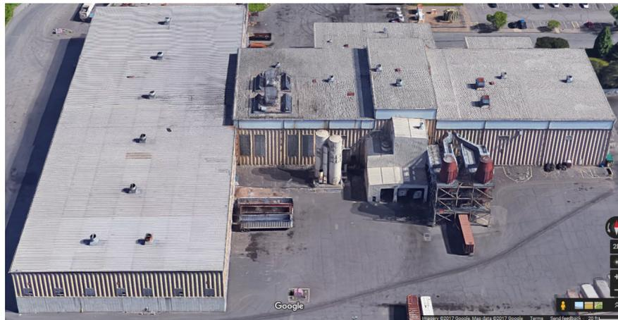
**The R&E Center:** A 1,500 ton-per-day resource recovery facility that shreds and separates trash to create value-added products. Trash is tipped by haulers onto a floor the size of a football field, and is fed into two processing lines that shred and sort the trash. The Center recovers metals for recycling, and produces refuse-derived fuel (RDF), which is currently used by power plants to generate enough electricity to power 28,000 homes.
